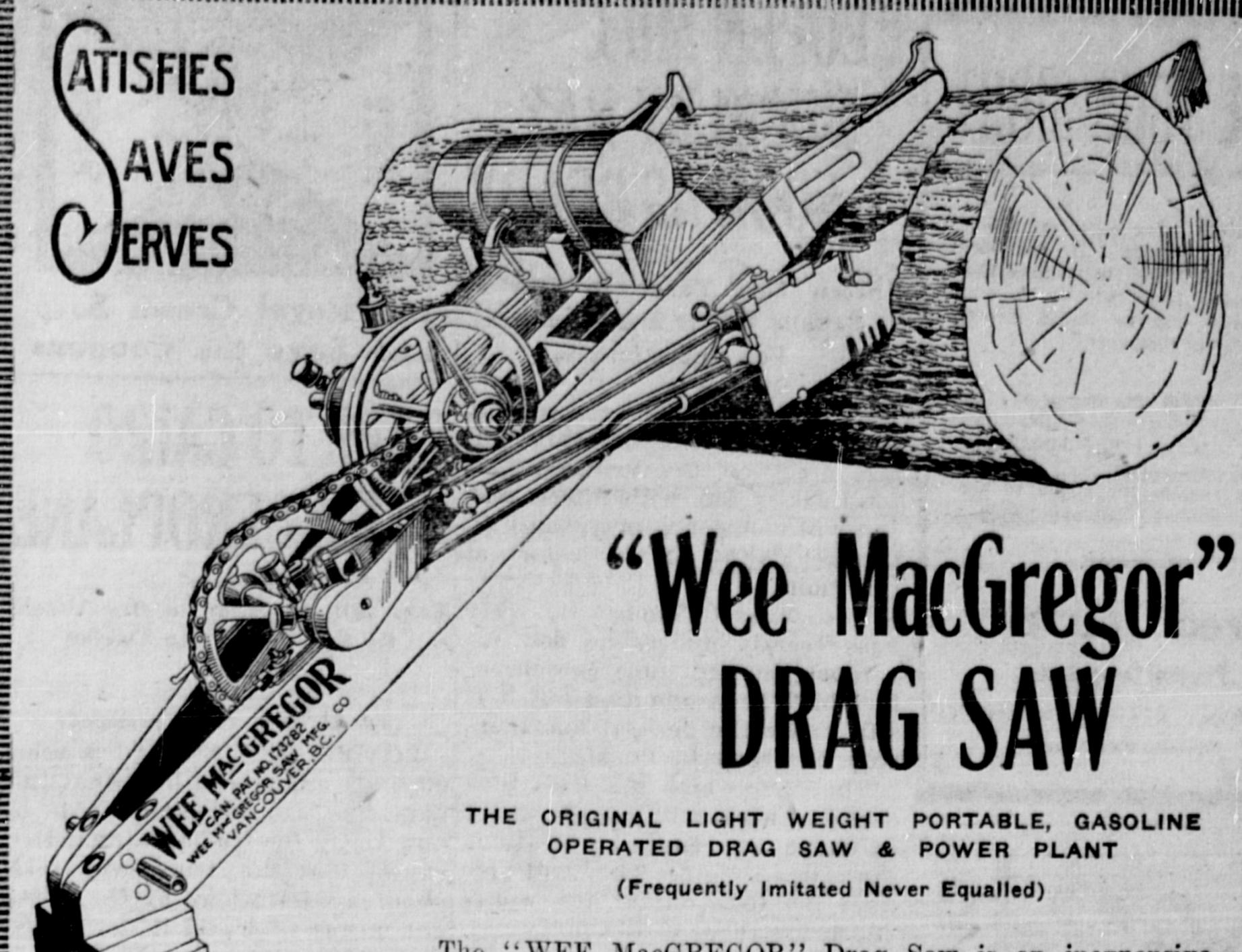
The "WEE MacGREGOR" Drag Saw is an inexpensive practical and proven machine, peculiarly adapted for the rapid and accurate cutting of wood under any conditions, on land or water. With equal facility and proportionate rapidity it will cut the small or large log up to seven feet in diameter. Depending upon size and character it will cut from either
