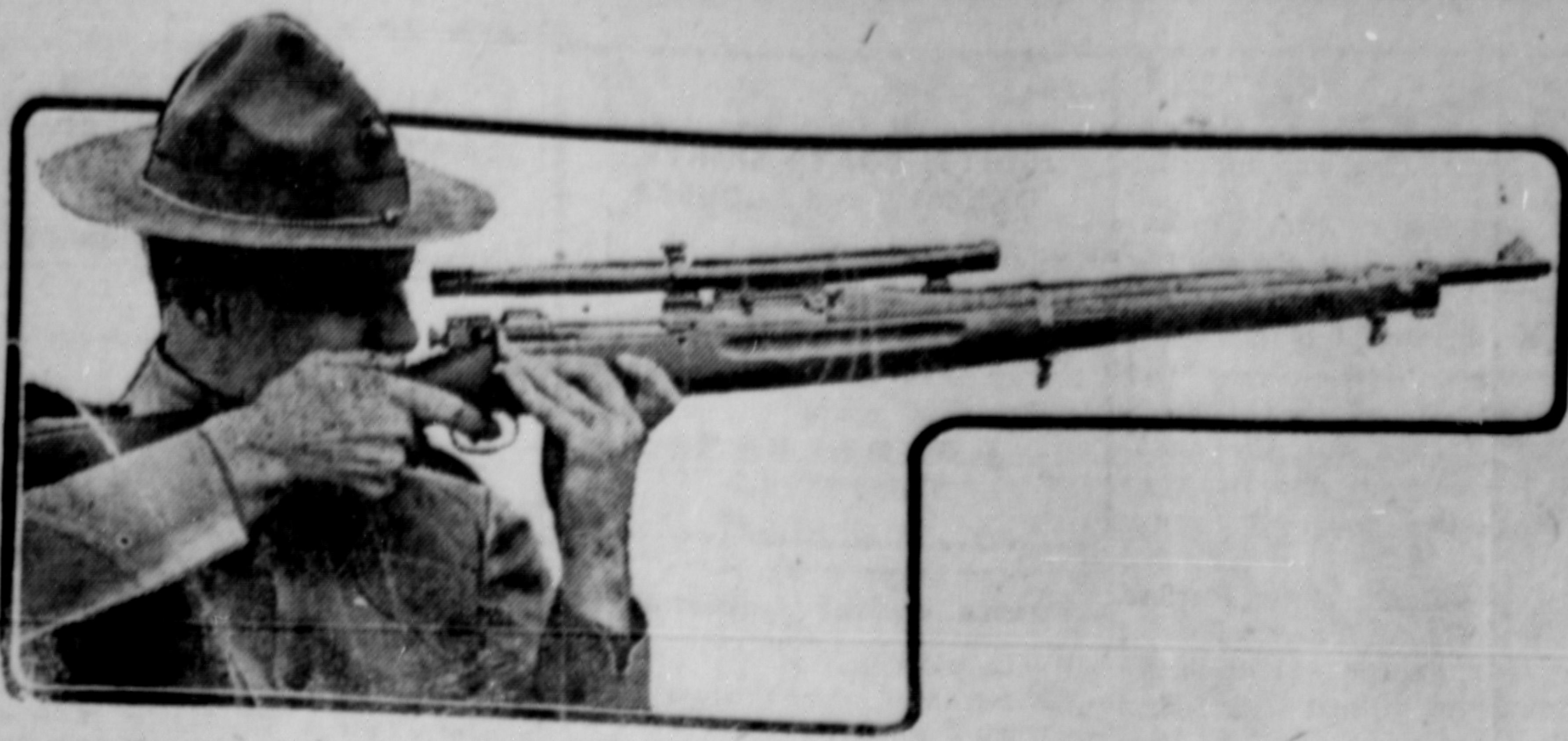
TELESCOPE SIGHT LATEST RIFLE DEVICE. —The Quartermaster's Department of the United States Marine Corps is trying out the new telescope sight for regulation Springfield rifle with a view to adopting it for this branch of the service. The sight is easily detached. It is for long range firing.
