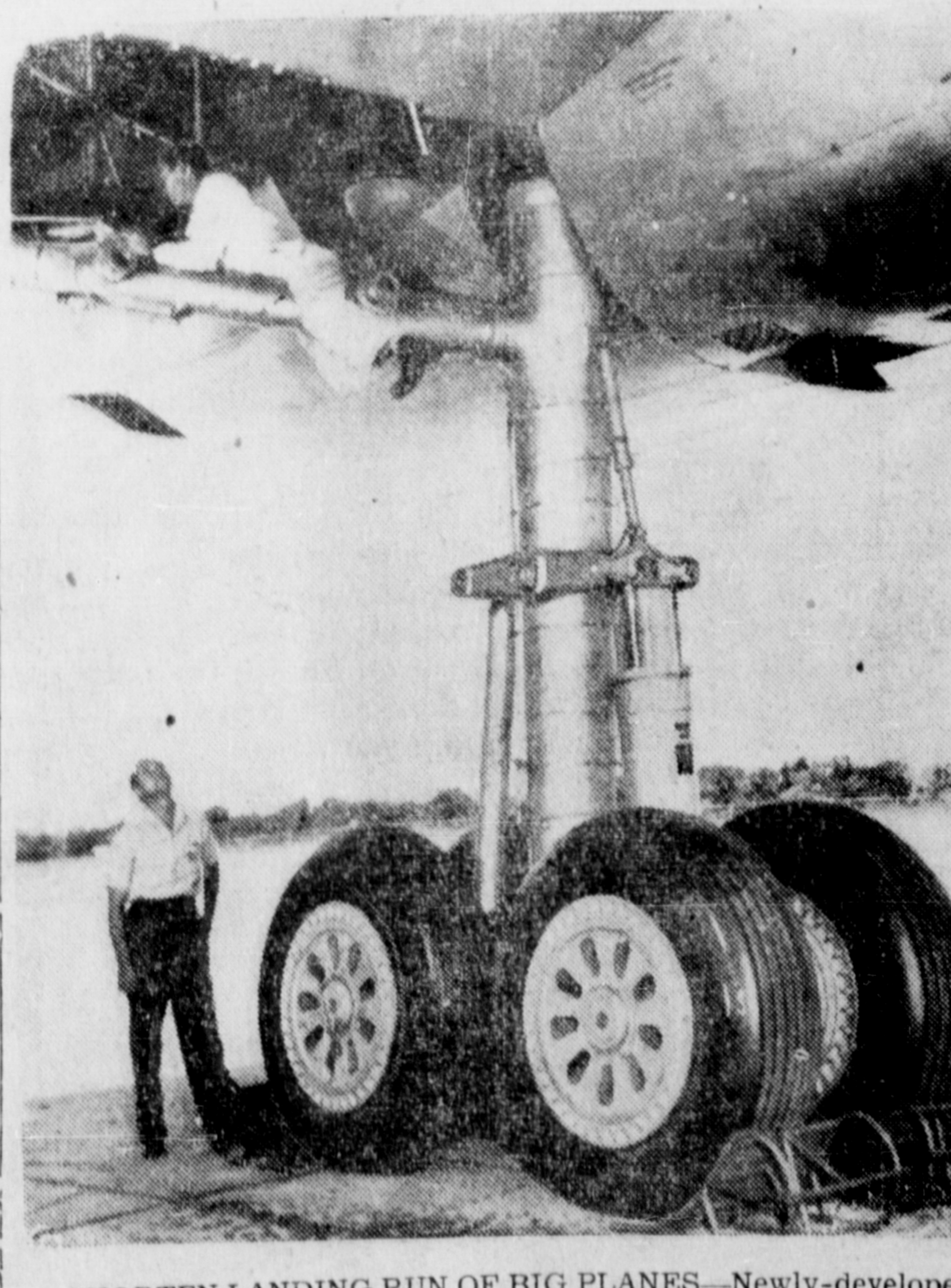
SHORTENED LANDING RUN OF BIG PLANES—Newly-developed four-wheel main landing gears are being installed on production-model B-36 super bombers at a San Diego airplane plant. The eight 56-inch wheels distribute the bomber's 278,000 pounds over a greater area than on two wheels and this weight distribution, coupled with shortened landing runs resulting from reversible-pitch propellers, will enable the giant six-engine bomber to utilize a greater number of airfields.
