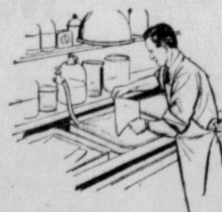
In the tanks, trays and washers used in processing black and white or color film, nickel alloys give high resistance to corrosion by developing and fixing solutions.
