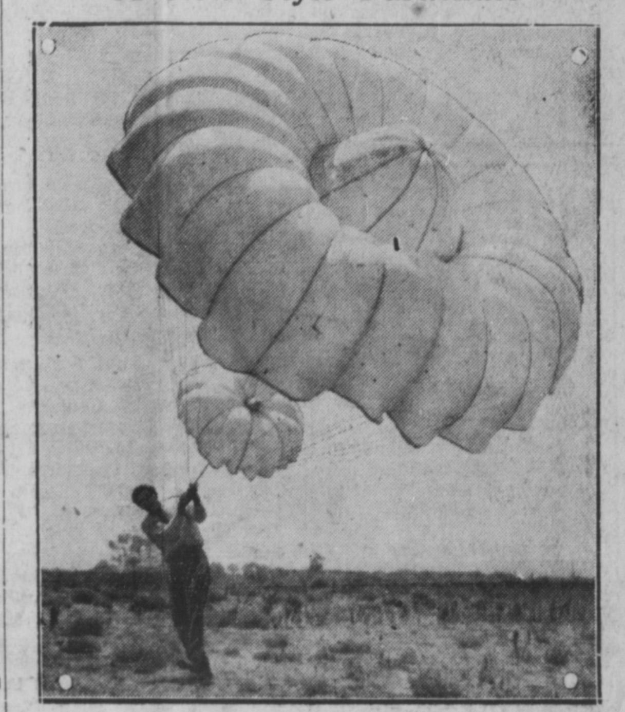
This new style parachute has been successfully tested in jumps from 45 to 3,000 feet. Its instancous opening is the feature and weighs less than 10 pounds packed.
