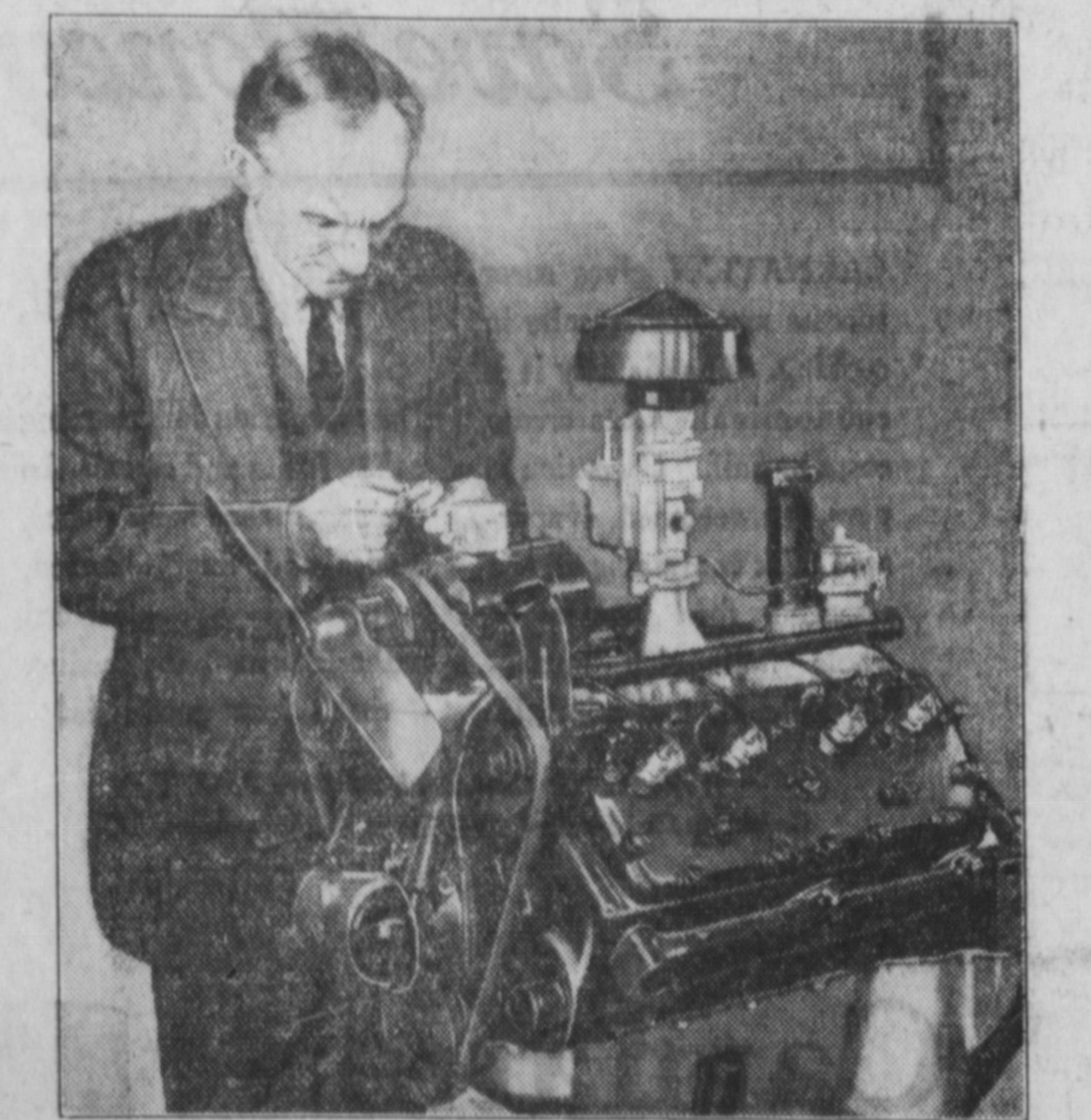
Photo shows Mr. Henry Ford at work on the new V-8 engine he created for the new Ford cars. The photograph was made in the Ford Engineering Laboratories at Dearborn, Mich. The photograph also shows the new engine, with its cylinder blocks set at 90 degrees; the fan, generator and two centrifugal water pumps driven by belt from the crankshaft; the distributor below the fan, and the downdraft carburetor and intake silencer, oil filler and crankcase breather pipe and fuel pump on top of the engine.
