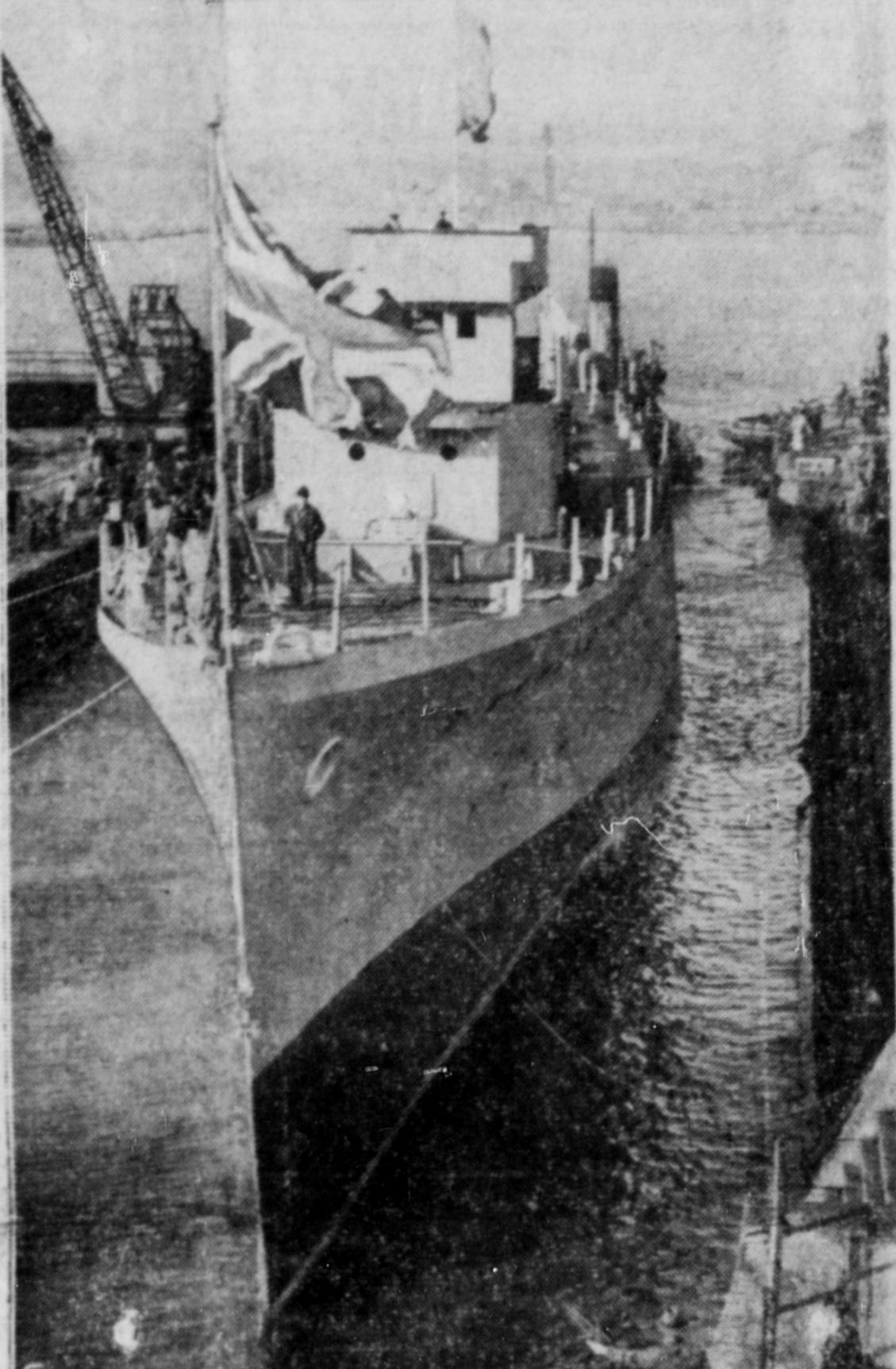
In keeping with the new British policy of heavy reararmament and the forsaking of disarmament conferences, the government launched this new 1,660-ton naval sloop at Chatham, England. The vessel is known as H.M.S. Deptford and is the latest of the "general service" class authorized under the 1933 program. She carries light armament and is an oil burner with 16-knot speed.
