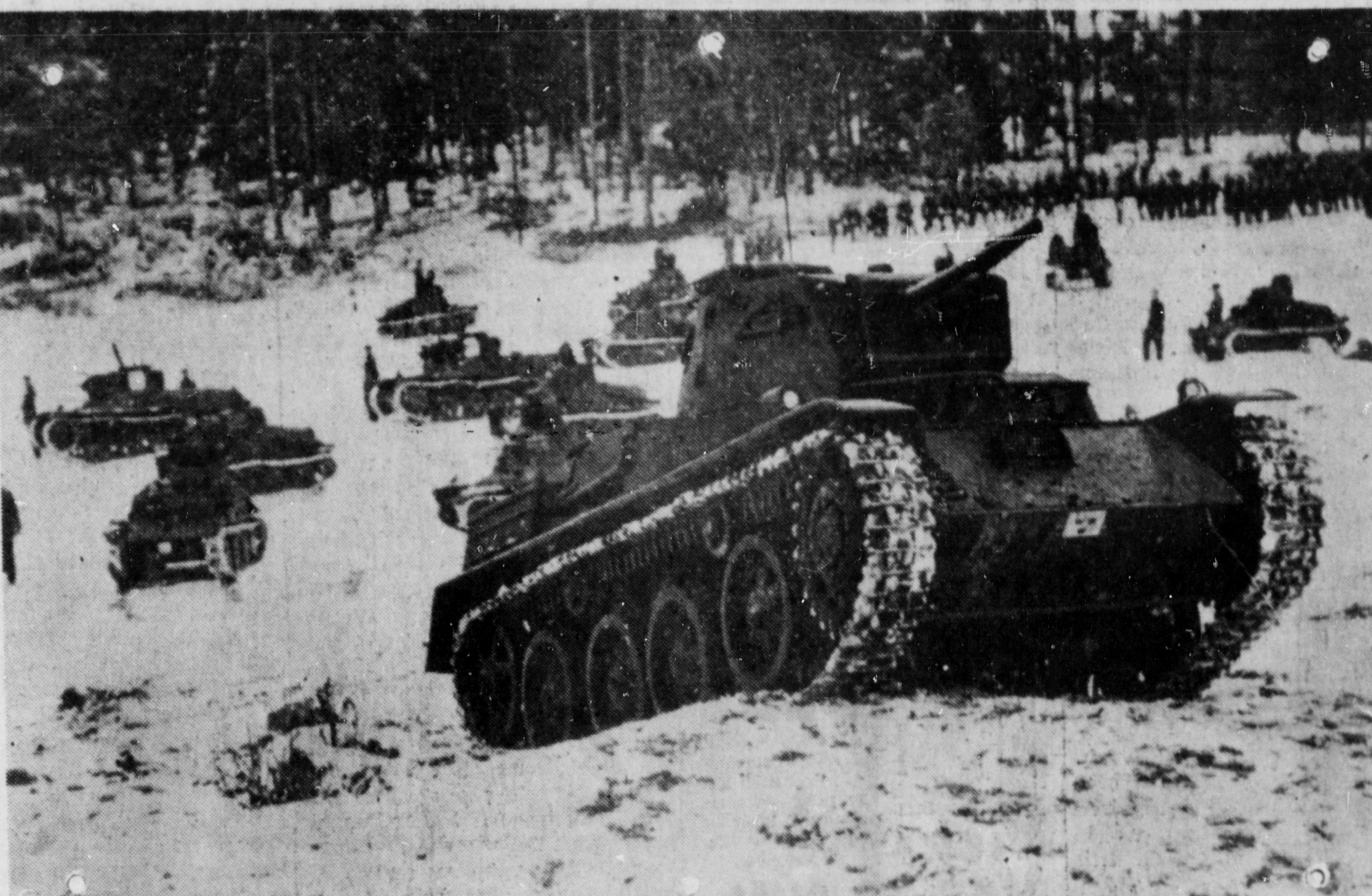
Sweden may be the home of the Nobel peace prize, but it is also equipped for meeting trouble if trouble is forced upon it. Here are some of the Swedish tanks that form a part of the defence force. These tanks, rated as among the world's most efficient, are equipped with two-way radio and can travel over rough terrain at 28 m.p.h. Swedish armament factories are acknowledged to turn out the best and most modern army equipment in the world, and it is ironic that much of Germany's armaments were made either in Sweden or from Swedish steel.
