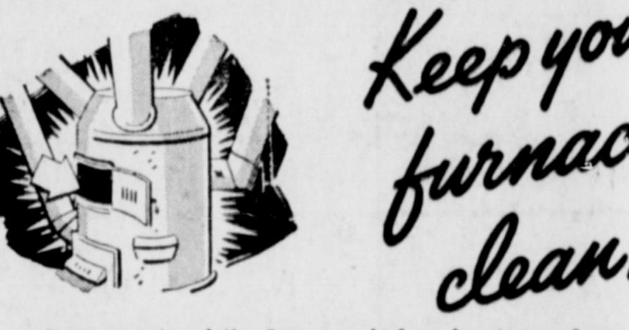
Remove ashes daily. Scrape scale from heating surfaces. Clean soot from smoke pipes and at base of chimney. You will have more heat and burn less fuel.
