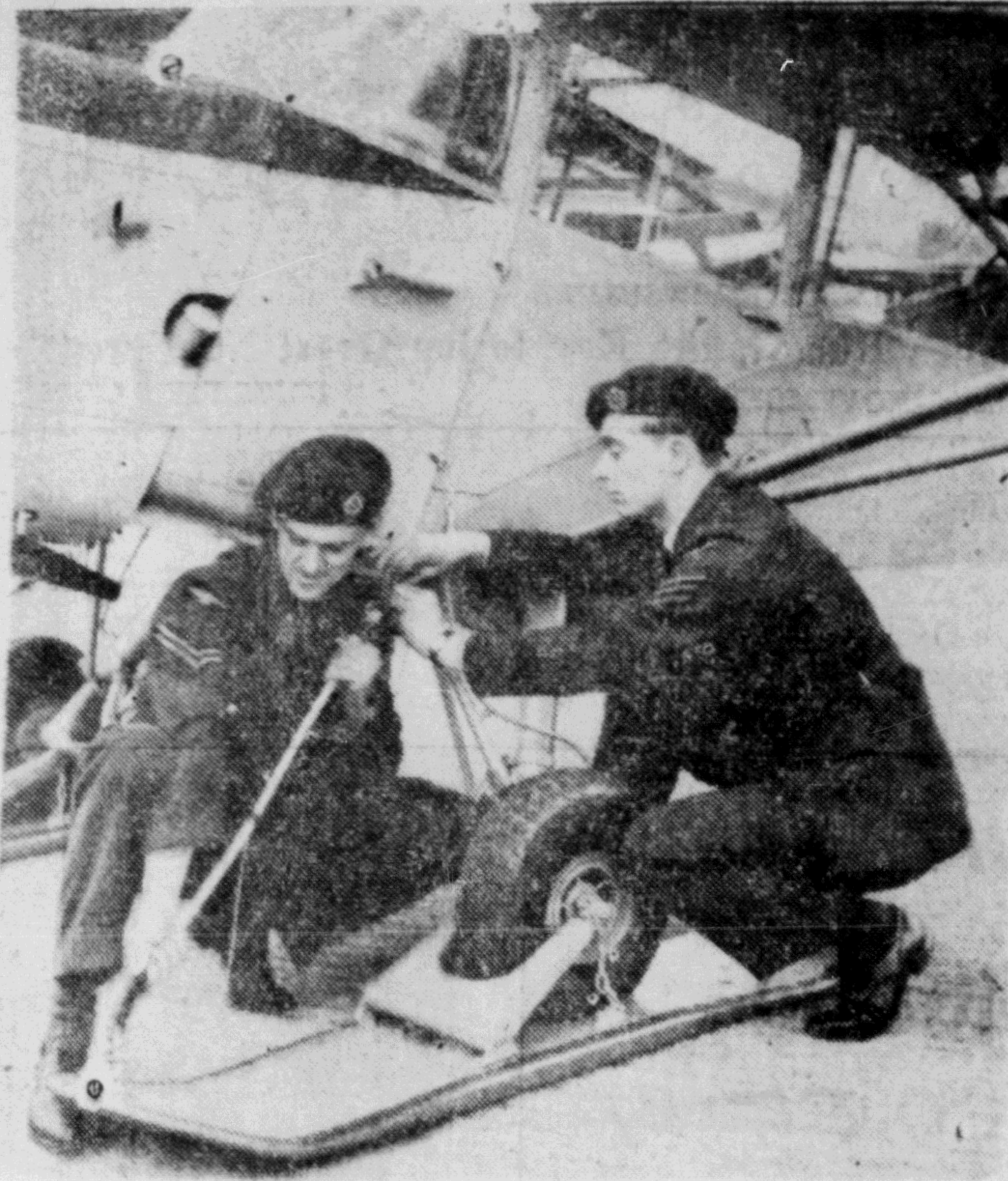
AIRCRAFT TO CONQUER ANTARCTIC—An R. A. F. Contingent and two specially adapted Auster Mk. 6 ski-equipped aircraft will be in the joint Norwegian-British-Swedish scientific expedition that will set out for Queen Maud Land, an unexplored tract in the Antarctic, in November. Difficulties of pack ice helped defeat the Shackleton expedition of 1914, but aircraft may overcome this difficulty by performing reconnaissance in the search for a passage by the members of the R. A. F. unit, Cpl. W. G. Gibbey and Sergt. P. D. Weston, make a last-minute adjustment to the special skis for landing on the snow-bound Antarctic mainland.
