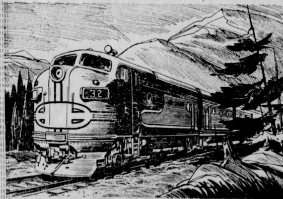
In the new diesel electric locomotives Nickel Steel gives greater strength with less weight. Steam locomotive boilers are made of Nickel Steel—tough, strong and durable at high temperatures.
