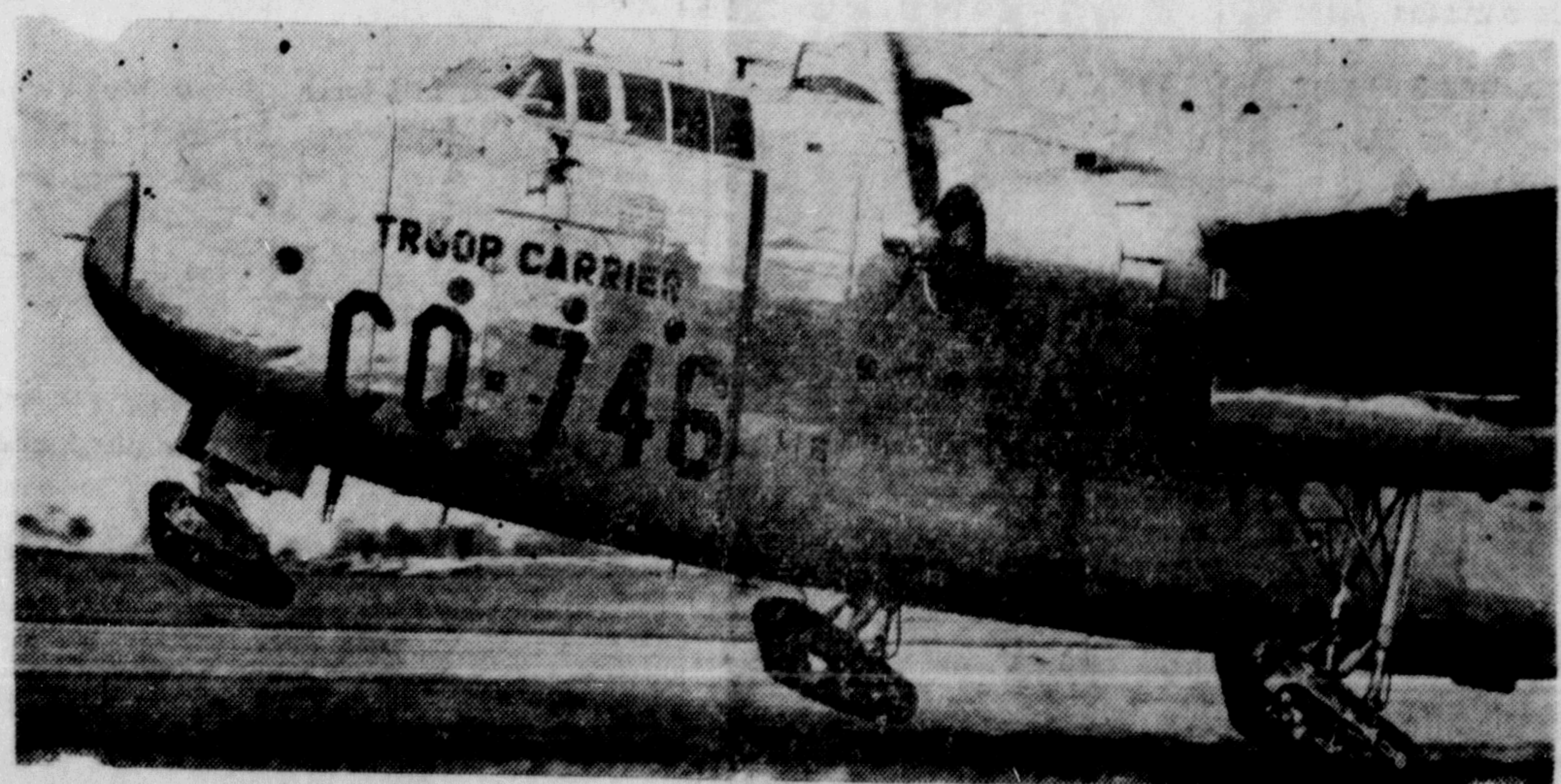
FIRST AIRCRAFT TO BE EQUIPPED WITH TRACK-TREADING GEAR —An air material command C-82, the first aircraft of any type to be equipped and flown with tricycle track-tread landing gear, settles on the runway following an early test flight at Hagerstown, Md. The track-type gear performs the same action as tank treads and permits landing on soft sand, mud or sod.
