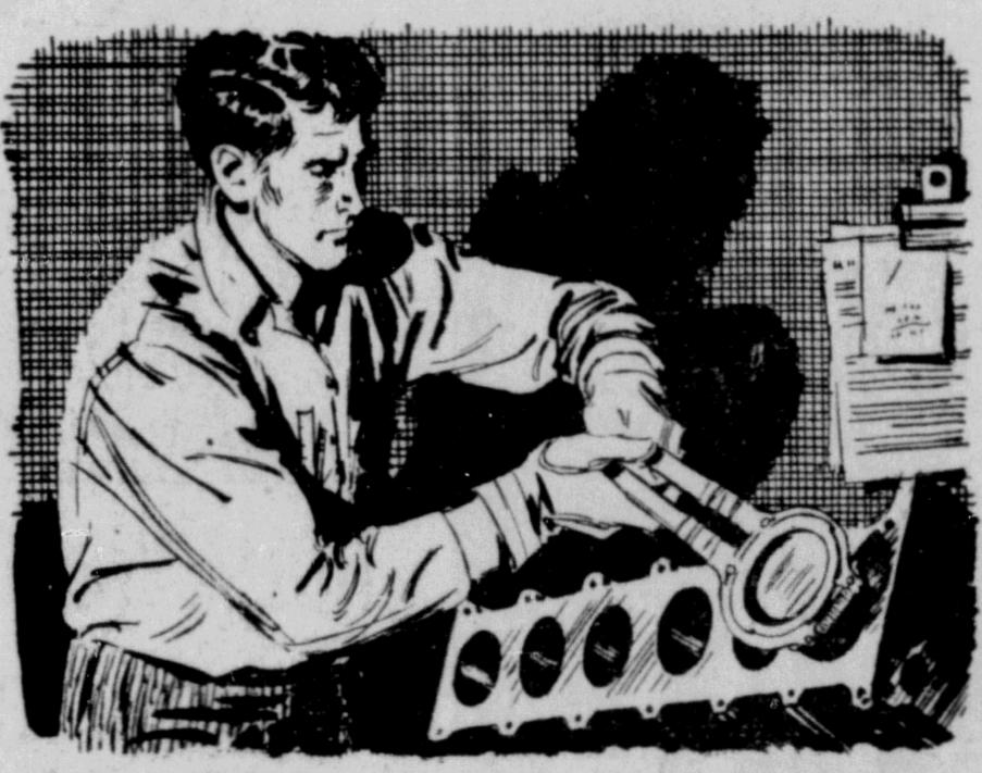
1. New atomic tool! Our scientists equipped test engines with piston rings treated at the Atomic Energy Commission's Oak Ridge Plant. For the first time, science measured wear as it happened!
