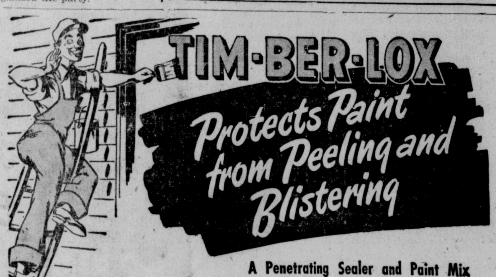
Tim-Ber-Lox is a clear liquid made from the finest, toughest resins and water-repellent oils and is used as a thinner for oil based paints or as a clear primer before painting or varnishing.
