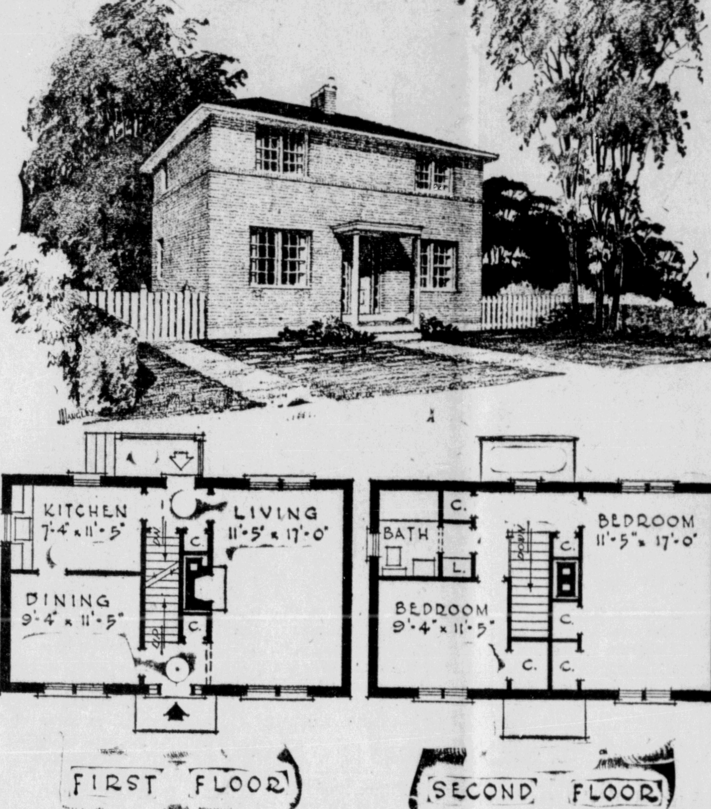
Although this Colonial type house is not large, its simplicity of line creates a dignified appearance. It is meant for a wide lot, with its wide frontage and fairly narrow depth. The perspective shows the exterior wall finish as brick veneer but the dimensions of the working drawings are so arranged that the house may be built of frame, brick veneer or solid masonry. The exterior dimensions are 30'10" x 18'8" and the total floor area for estimating purposes is 1,152 square feet.
