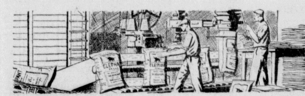
Because of seasonal demand for fertilizers, large storage space is necessary. Cominco's plant at Trail can store 100,000 tons. When required for shipping, fertilizers are placed in jute sacks or paper bags. Daily shipping capacity is over 2,000 tons.
