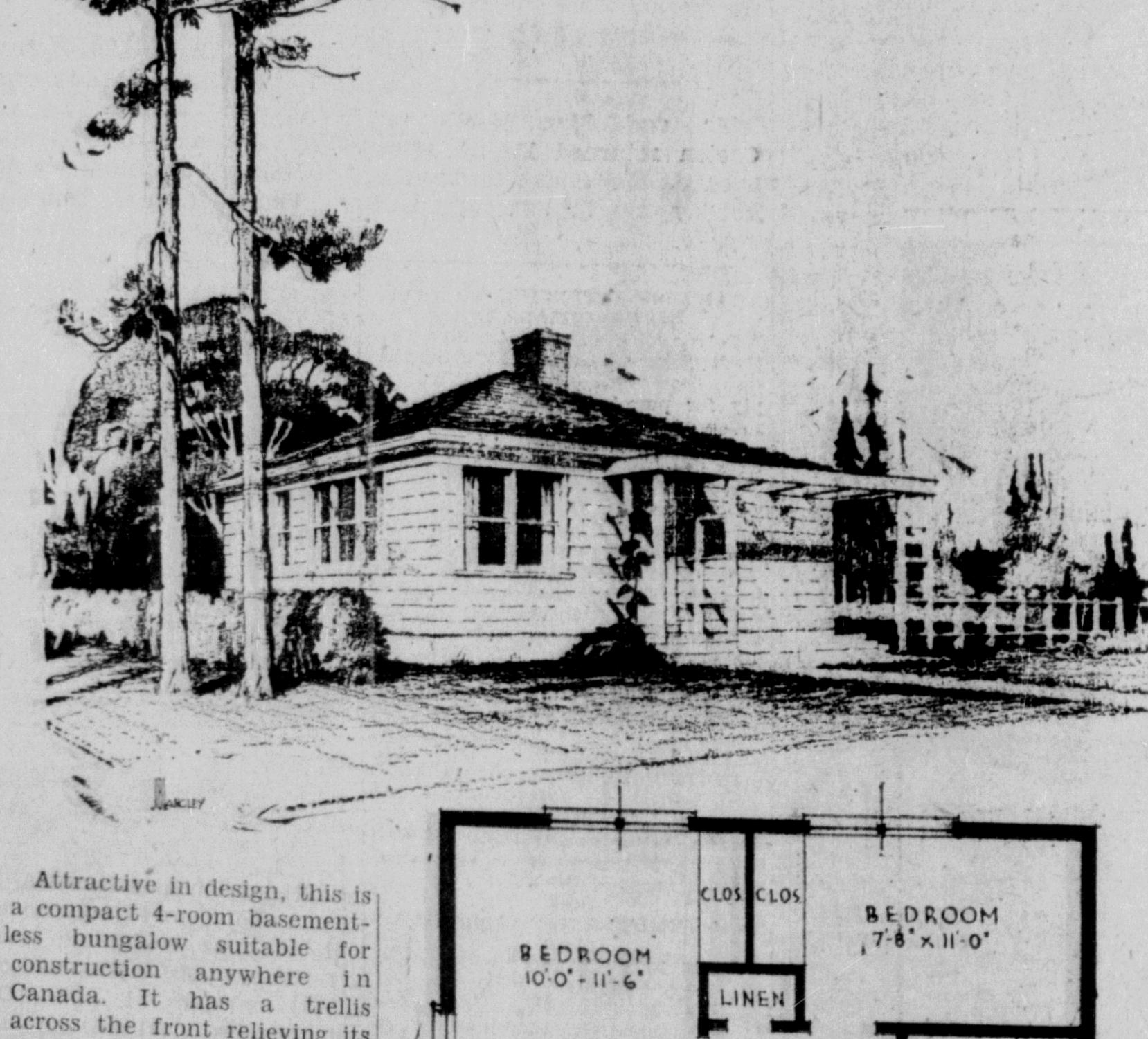
less bungalow suitable for construction anywhere in Canada. It has a trellis across the front relieving its simplicity. The exterior dimensions are 26' x 26' and' the area for estimating purposes is 676 square feet.
