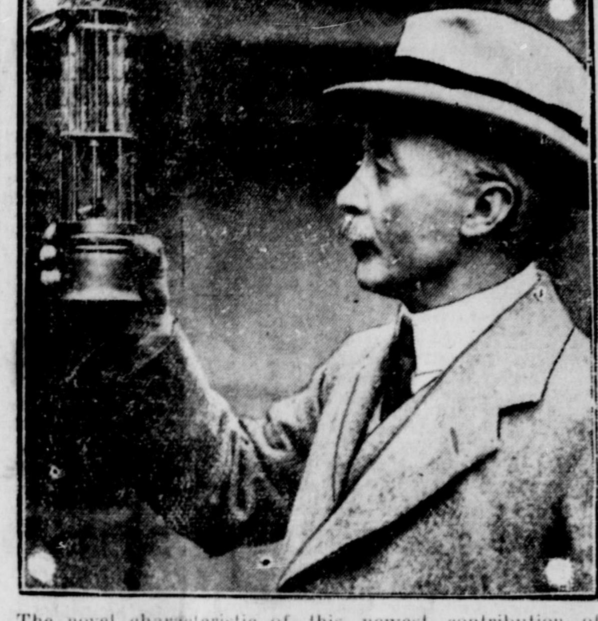
The novel characteristic of this newest contribution of safety in coal mines, is that it not only provided adequate means of illumination, but that it gives an audible indication when there is more than two per cent of fire damp in the working plant.
