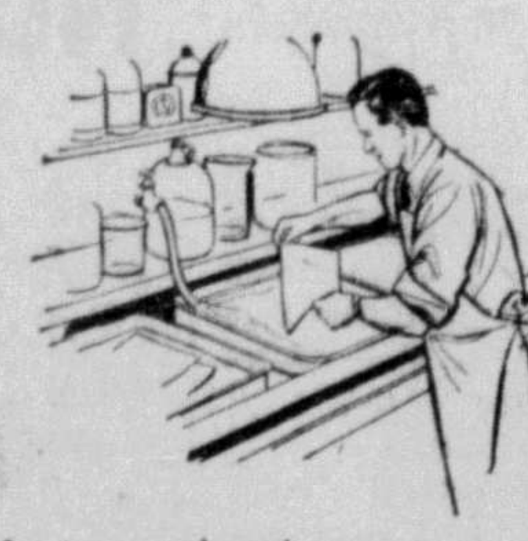
In the tanks, trays and washers used in processing black and white or color film, nickel alloys give high resistance to corrosion by developing and fixing solutions.
