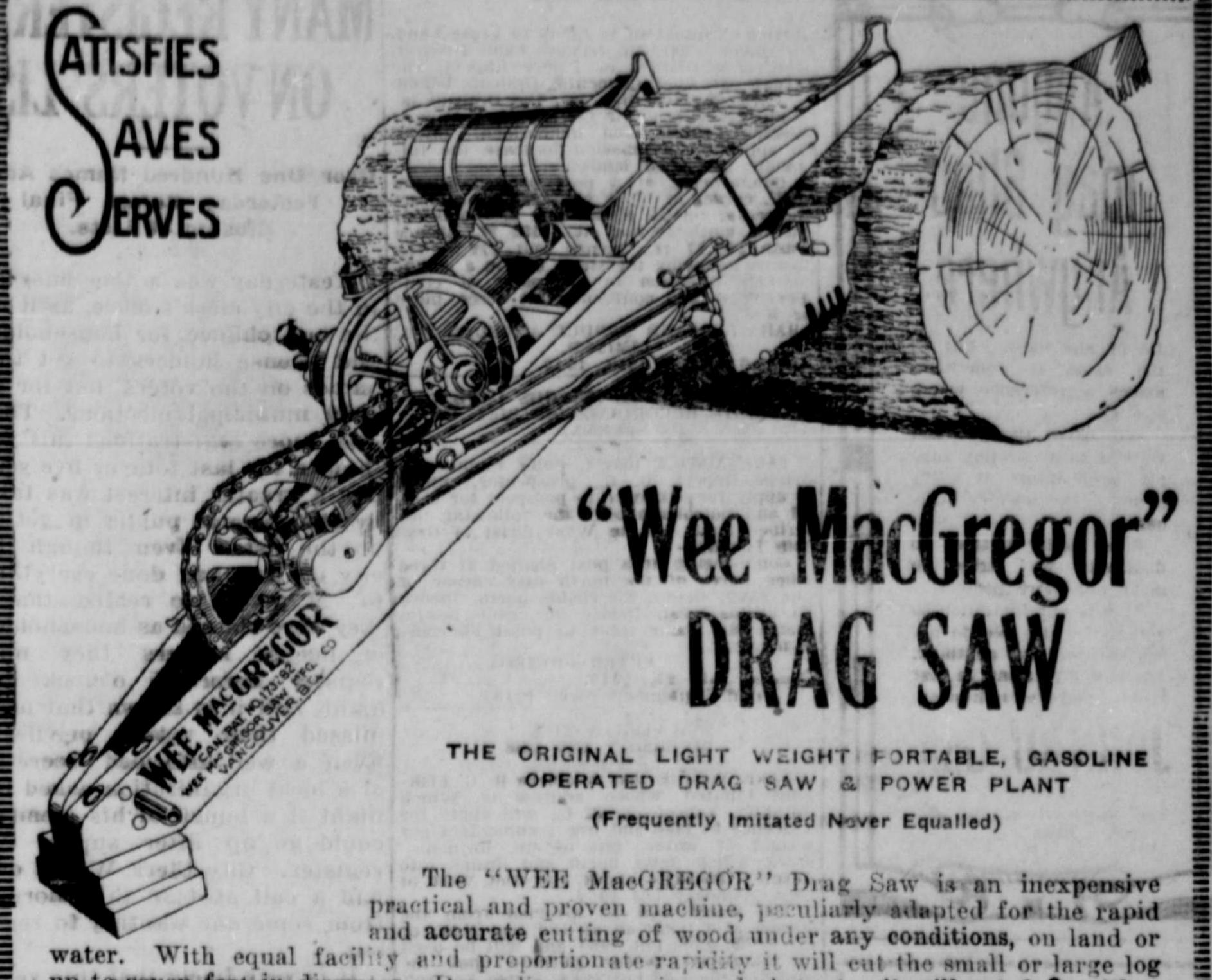
up to seven feet in diameter. Depending upon size and character it will cut from either green or dry logs, 20 to 30 cords of wood a day.
