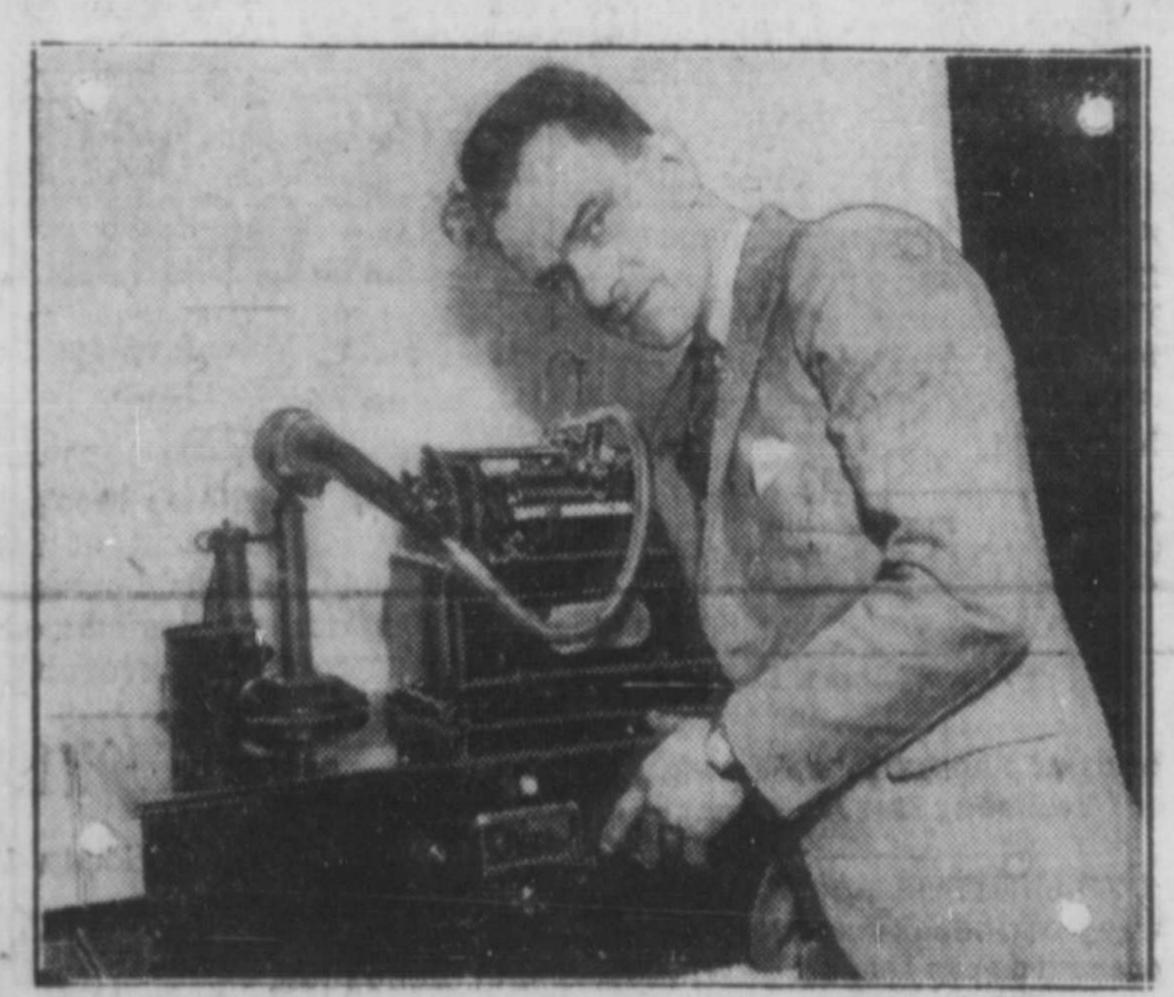
Newly-invented device which automatically answers telephone in absence of person intended has been invented by William Schergens of St. Louis. The machine operates by means of phonograph reproducing cylinders. Ringing of telephone bell automatically starts operation, setting machine in motion for message.
