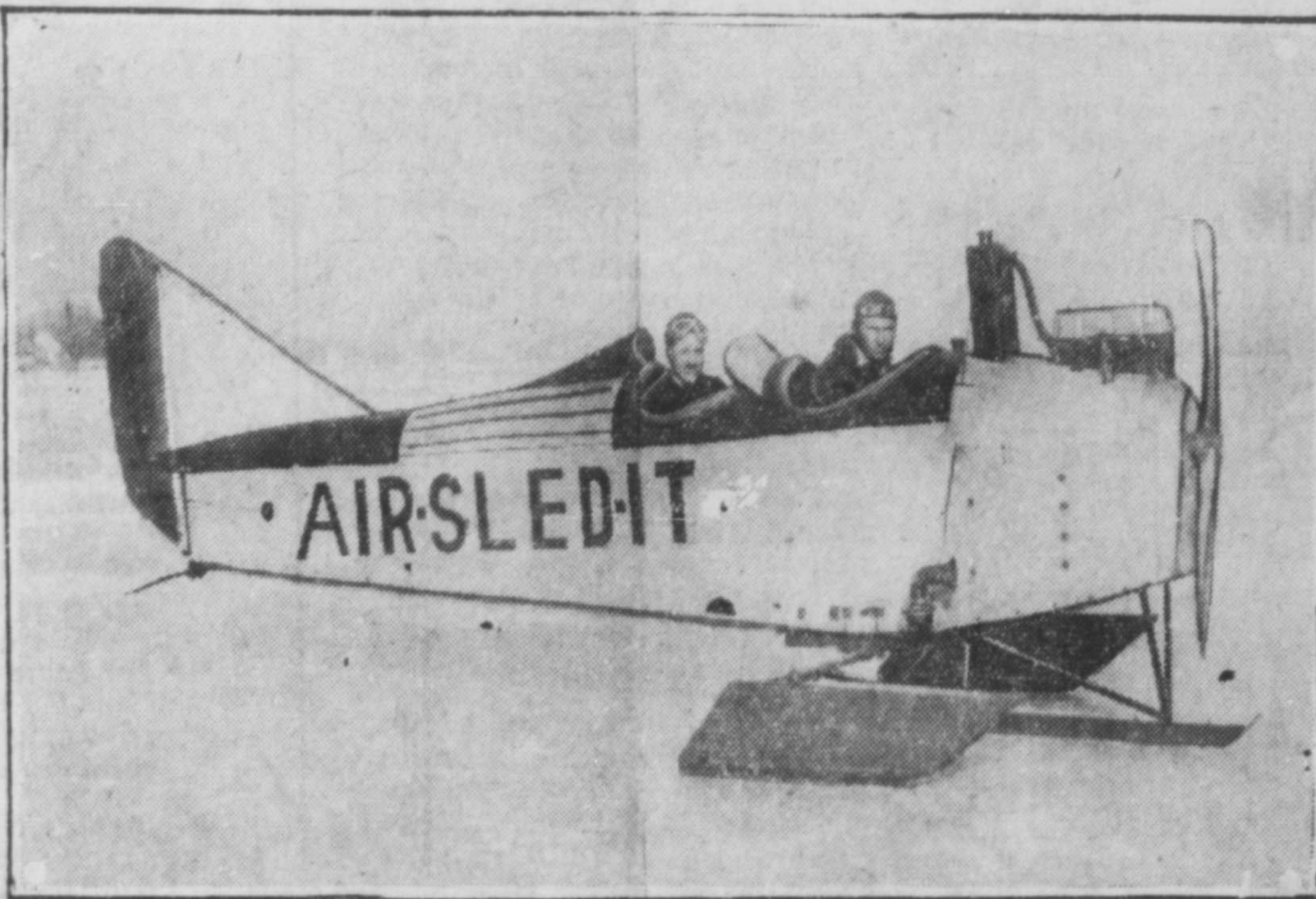
Shorn of wings, this old fuselage has been converted into a novel ice-sled with speed capacity of 75 miles per hour. Two youths in the cockpit Robert Ellwell and John Caldwell of St. Clair, Michigan, salvaged the machine after it had been in a crash.
