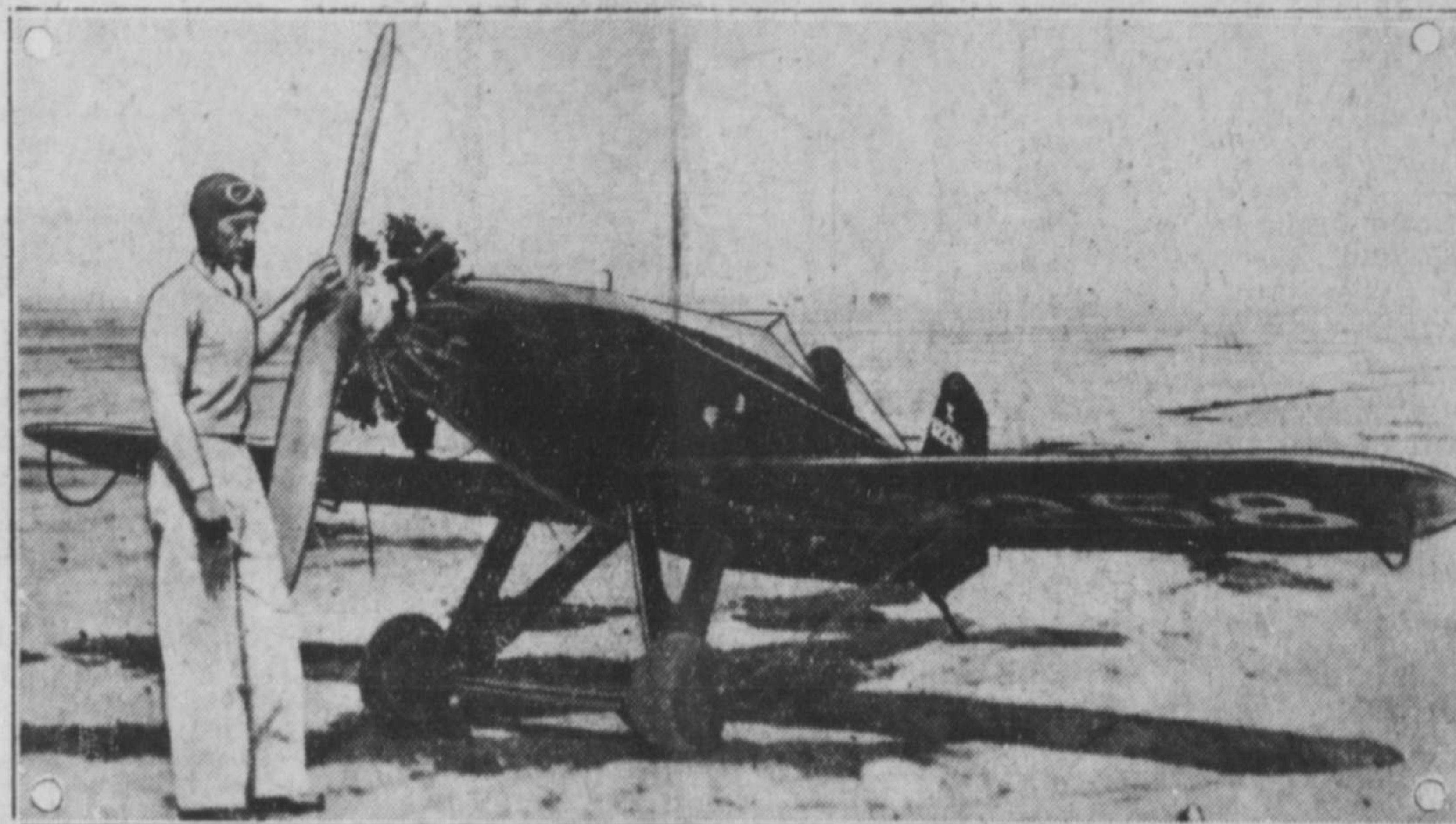
This is the "Doodle Bug," one of the smallest planes ever built for actual use. The wing is 20 feet long, the body 14 feet and a 40-horsepower engine gives it speed of well over a 100 miles an hour. George Hales, Californian, will compete at Cleveland in it.
