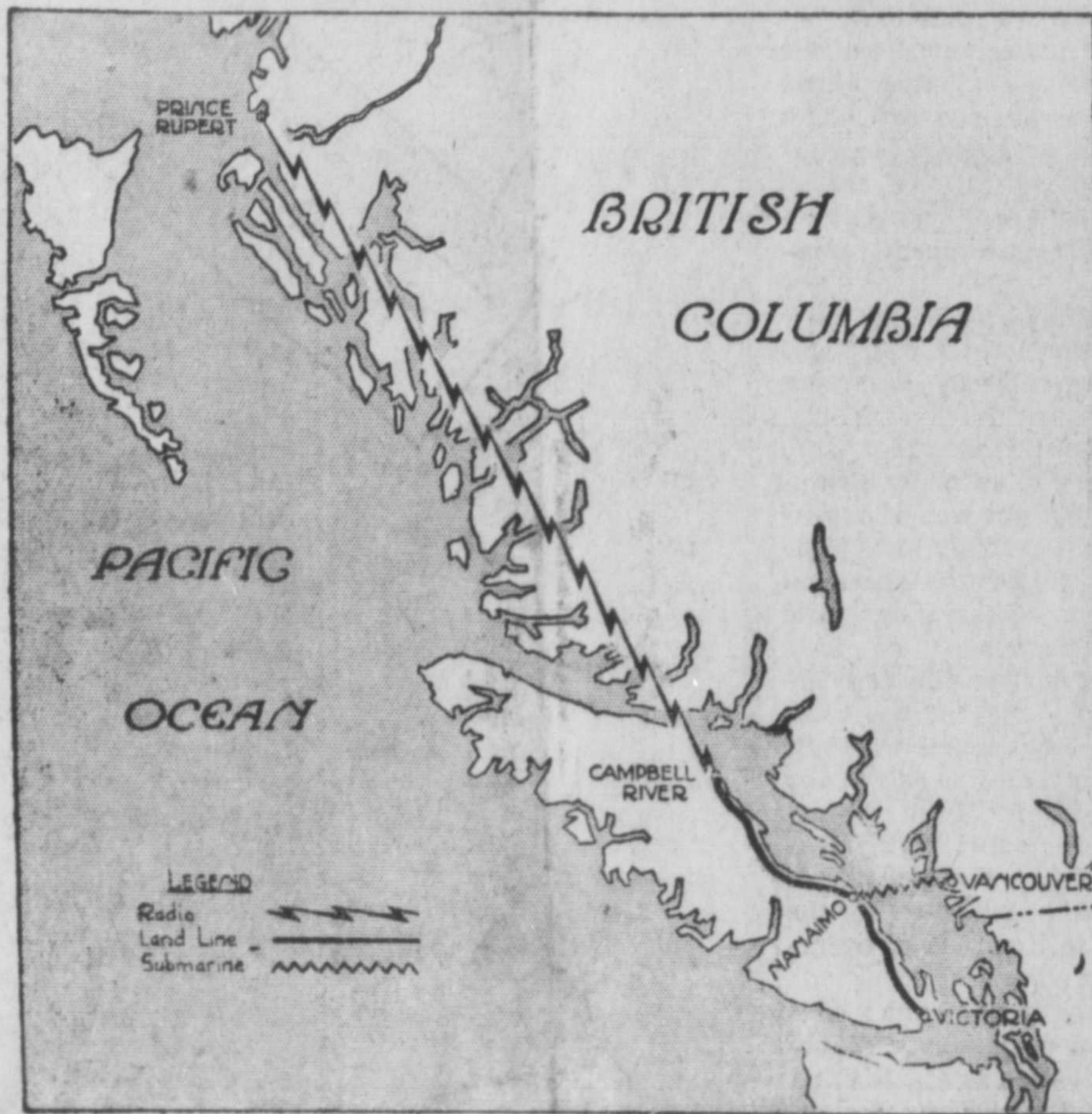
When talking by radio telephone with Vancouver, the voice is carried through the air to Campbell River 400 miles, then over 100 miles of land wire, 32 miles of submarine cable and 13 miles of ordinary cable.
