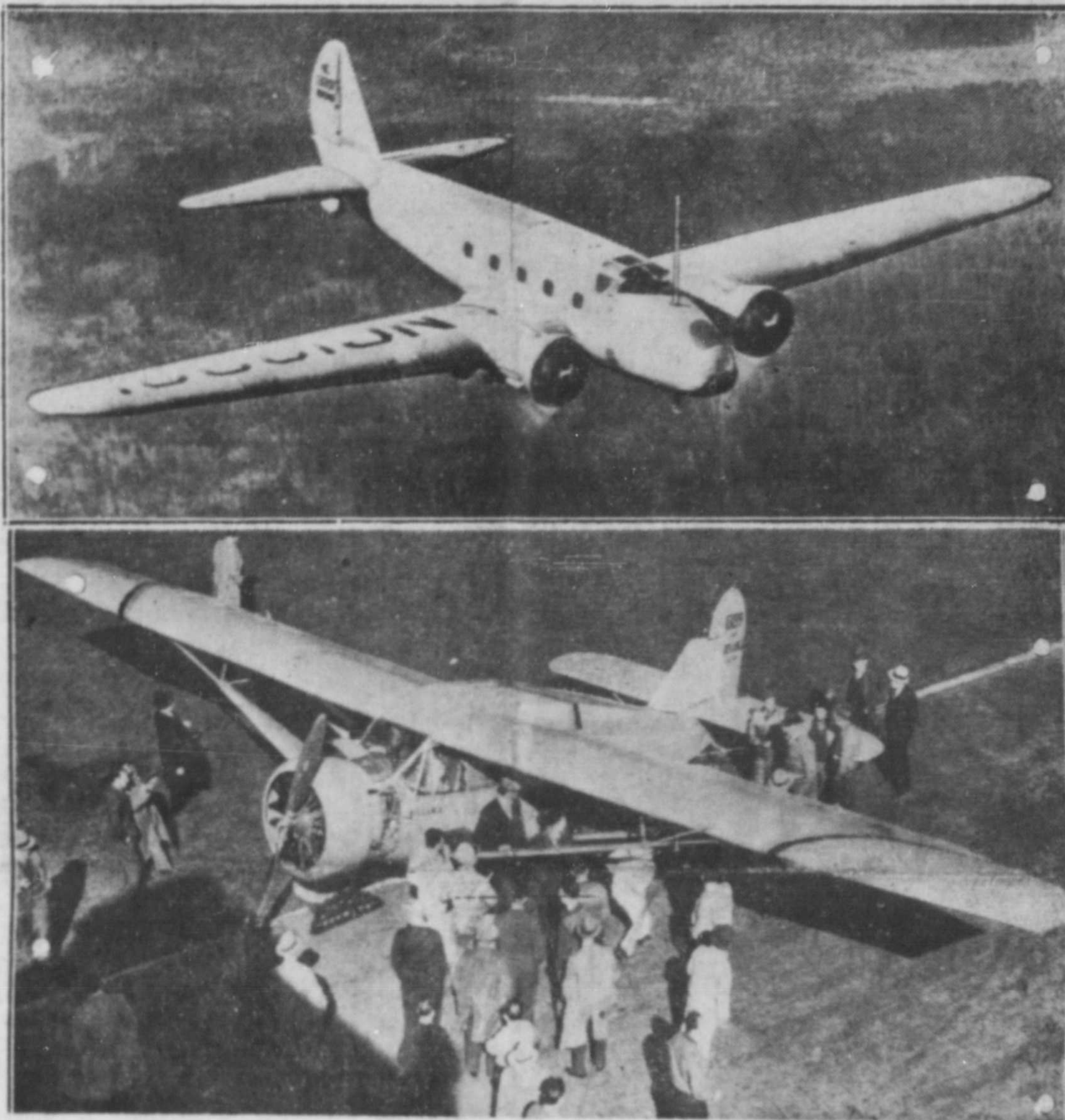
Upper photo—This new bi-motored, ten passenger aeroplane is being tested near Seattle. It has a top speed of 182 miles per hour and cruising speed of 165, wing spread of 74 feet and is powered by two 550 horsepower radial motors.
