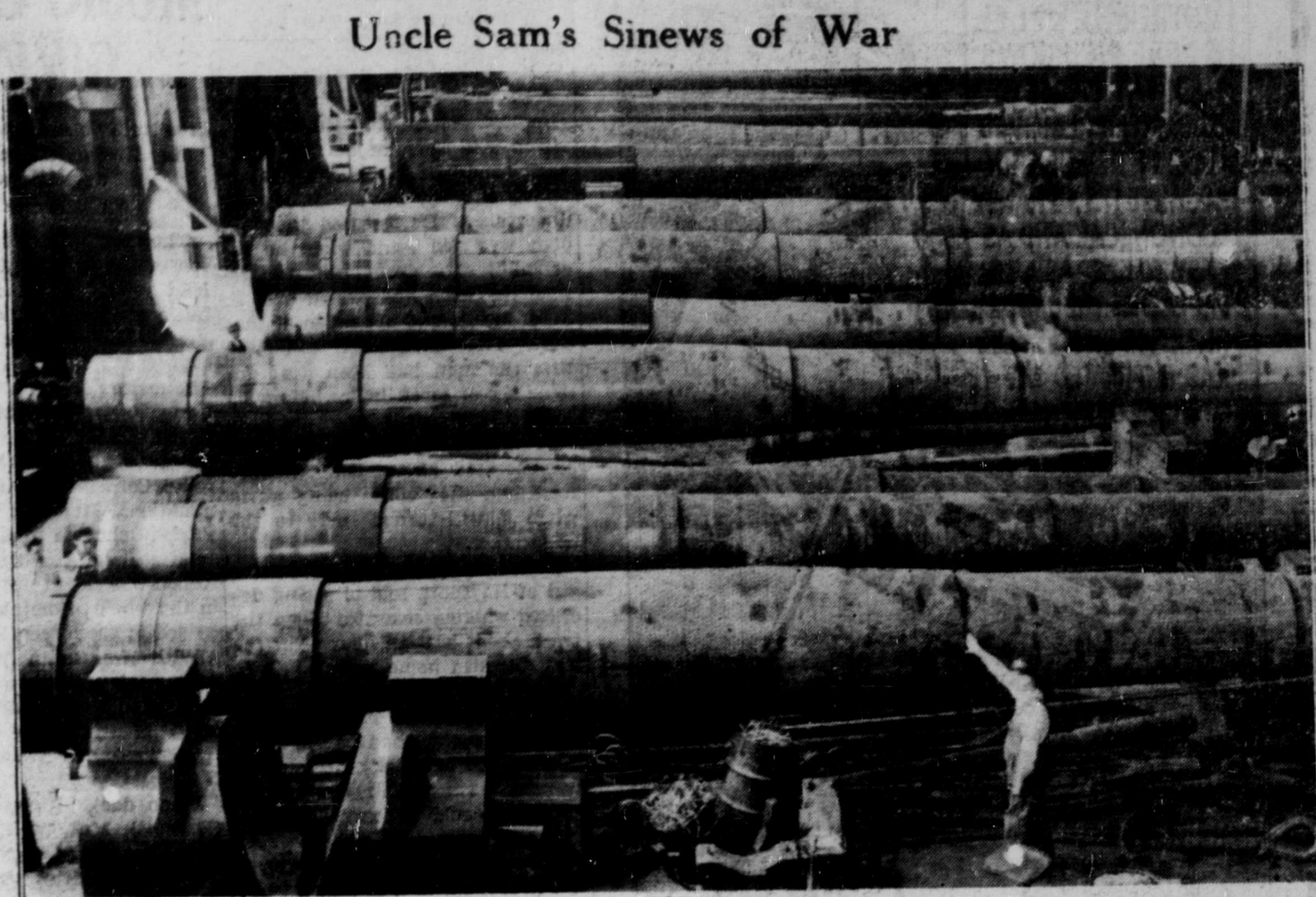
Fourteen and 16-inch dreadnaught rifles laid out for repair in the naval gun factory at Washington, D.C. The weapons have "throat trouble" and workmen hammer and chisel on them for 24 hours a day, getting them back into good condition.
