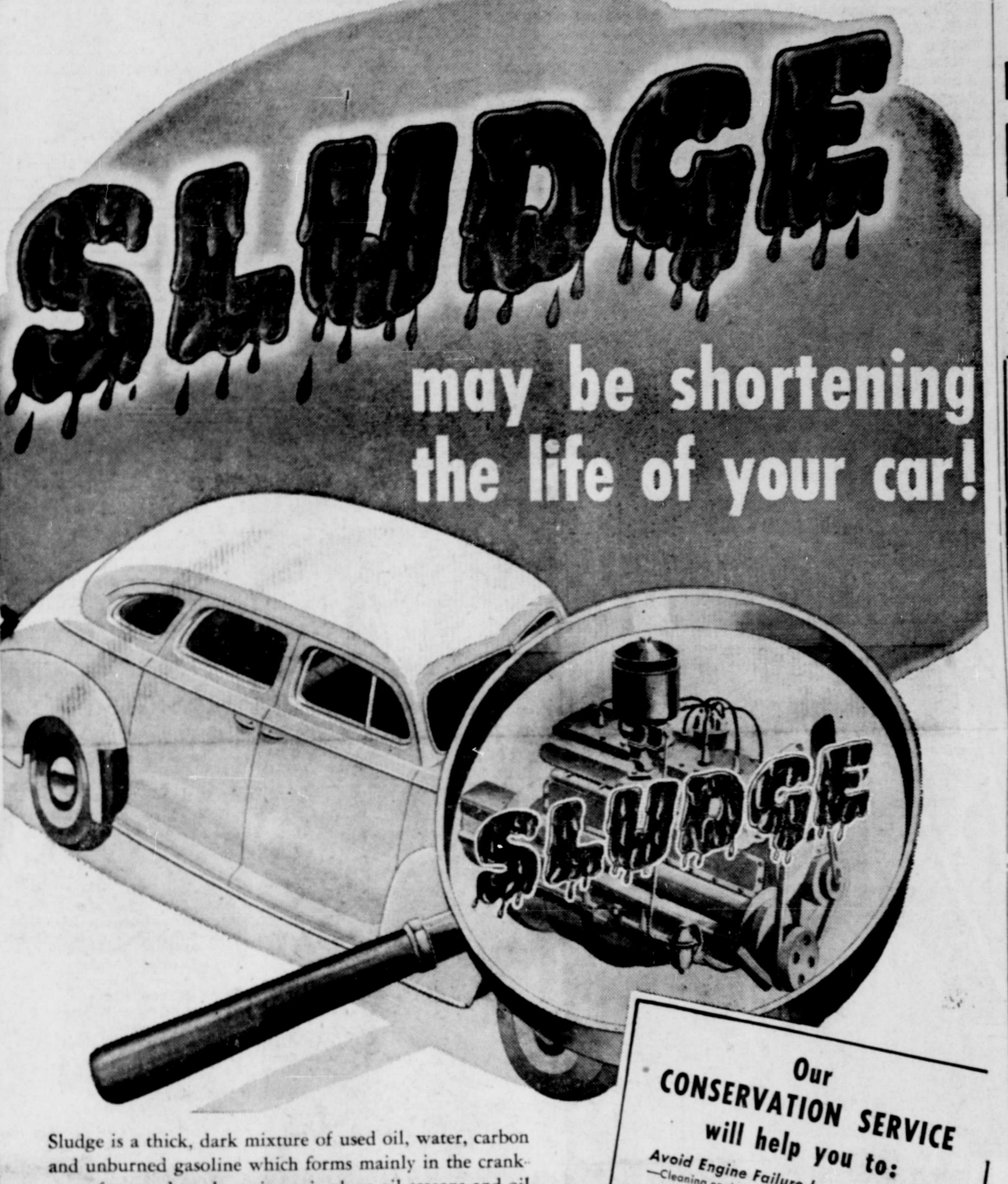
Sludge is a thick, dark mixture of used oil, water, carbon and unburned gasoline which forms mainly in the crankcase of car and truck engines-it plugs oil screens and oil passages and damages other engine parts.
