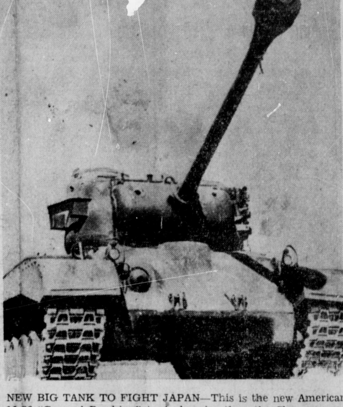
NEW BIG TANK TO FIGHT JAPAN-This is the new American M-26 "General Pershing" tank, heavier than the Sherman and with a lower silhouette. Its high velocity 90 mm. gun can knock out enemy tanks at ranges of two miles or more. The poweroperated turret, improved fire control, and interior arrangements make it capable of delivering accurate fire at a greatly increased rate, while thickness and slope of the armor provide maximum protection.
