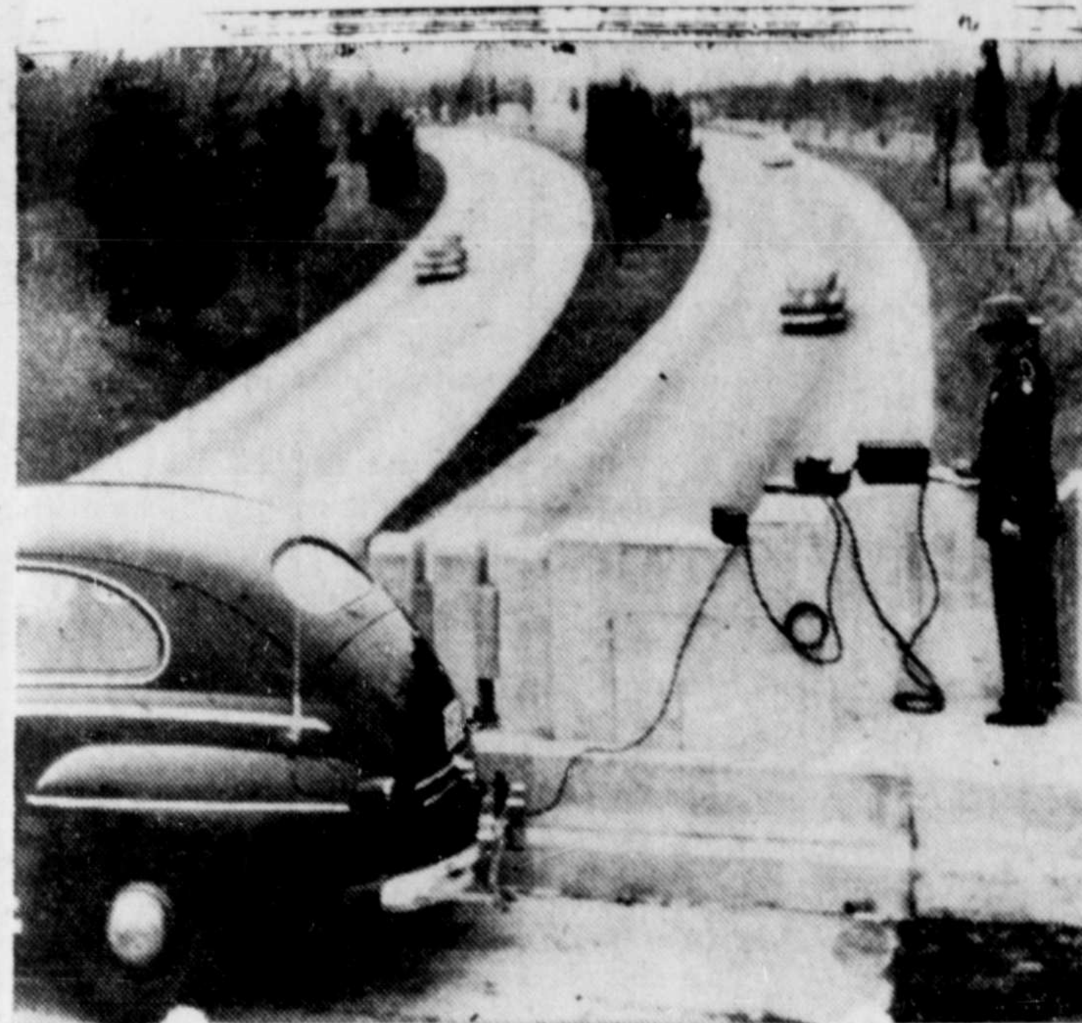
SPEEDERS BEWARE OF RADAR —Standing beside a radar device that will be used on Connecticut roads to cut down on speed motorists is one of the state troopers now learning how to operate the new gadget. Known officially as the electronic speed meter, it can compute the m.p.h. of cars as its wartime cousin figured the speed of approaching planes.
