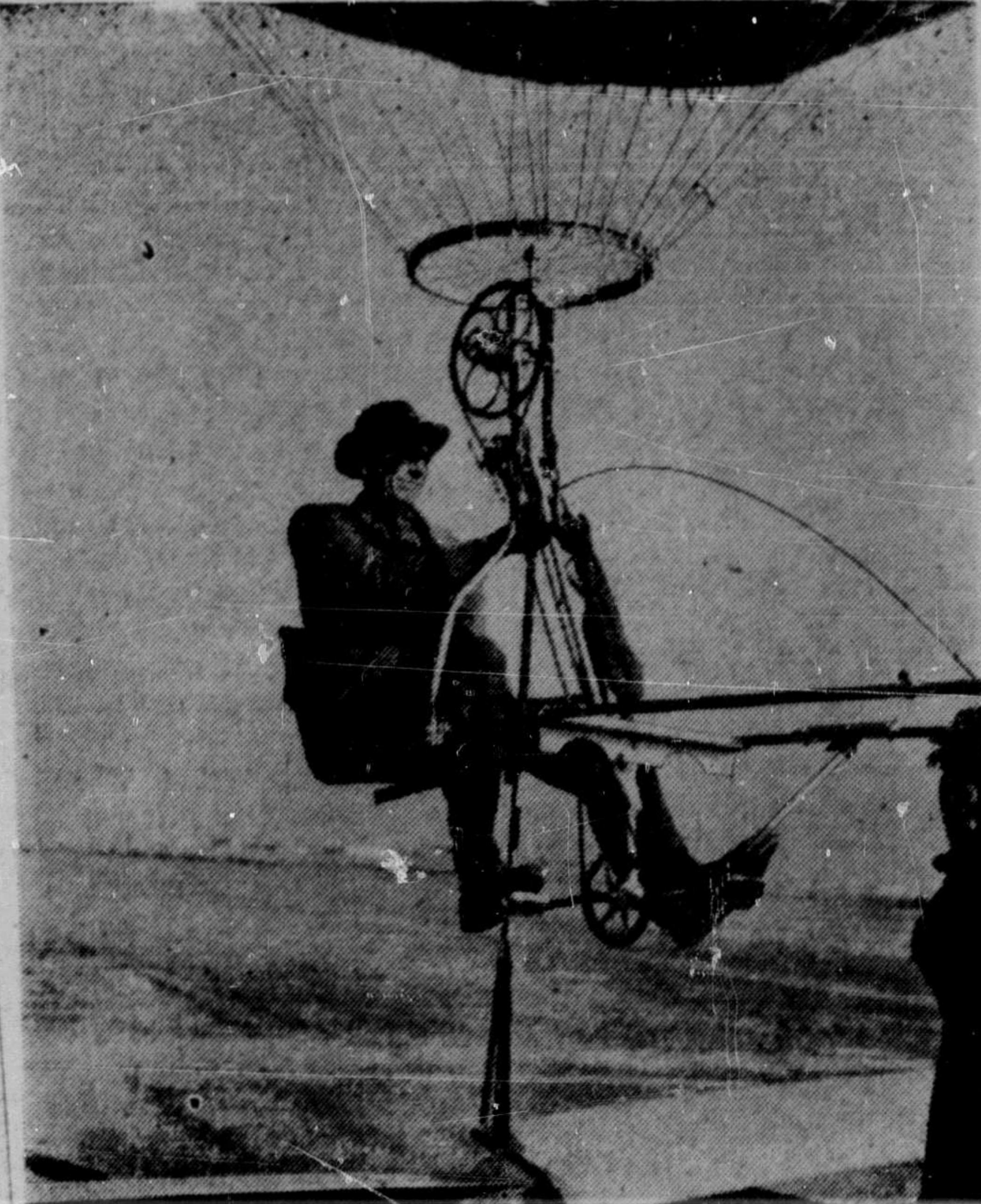
MUSCLE POWER MOVES PEDALCOPTER AT 10 M.P.H.—Navy Attorney Charles Paul is shown at the controls of his Pedalcopter at Lakehurst, N. J. The novel machine weighs 140 pounds and has a 24-foot balloon. The machine has no engine, but ascends on power supplied by the pilot. The pilot sits in a frame suspended below the balloon and uses a bicycle device to drive the helicopter blades and operate the craft.
