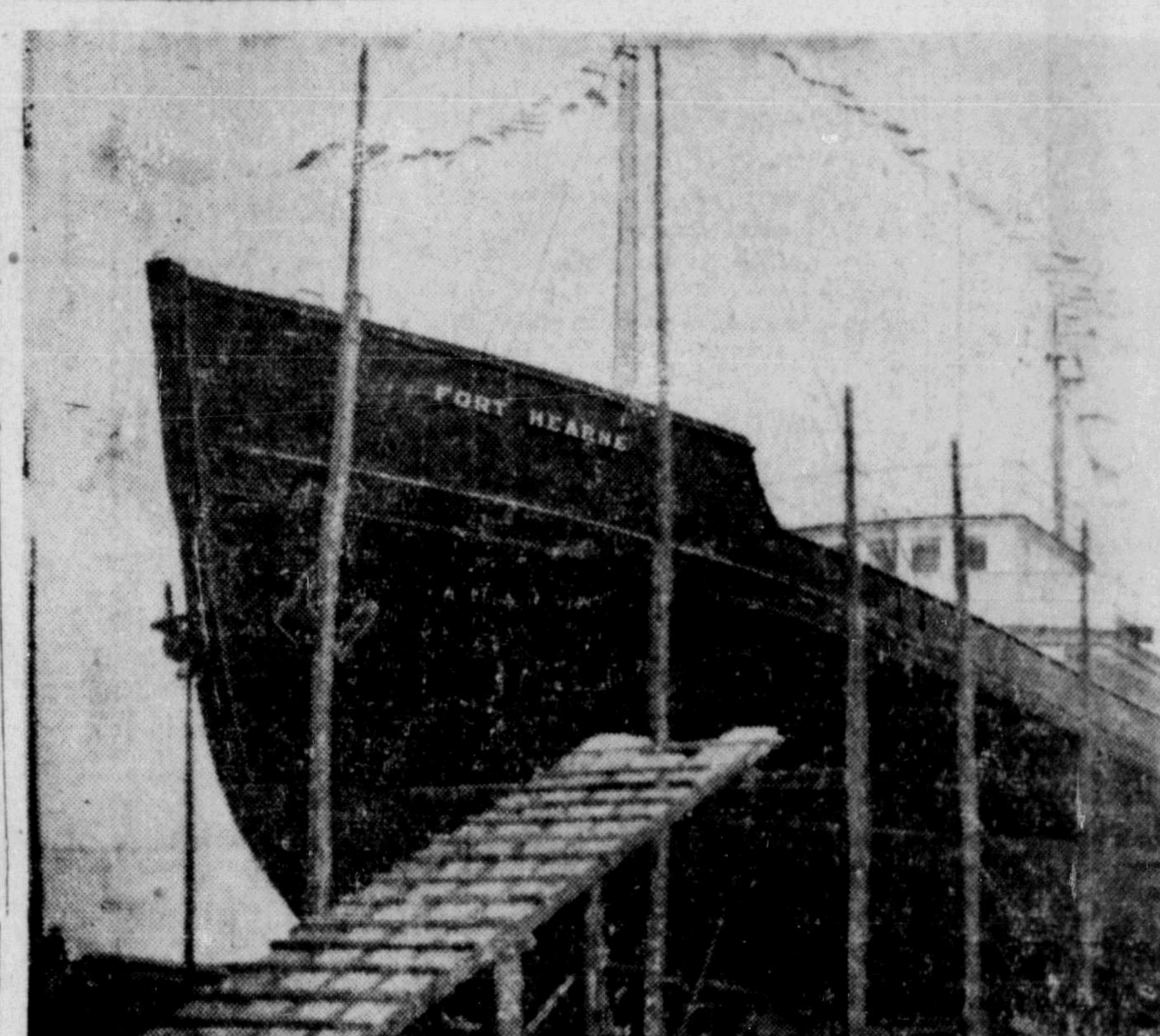
ARCTIC FREIGHTER—The Fort Hearne, shown here prior to being launched in N.S., will become part of the Arctic fleet of the Hudson's Bay Company when one of the largest wooden ships built in the Maritimes in years, the vessel has an overall length of 149 feet with a 30-foot beam.
