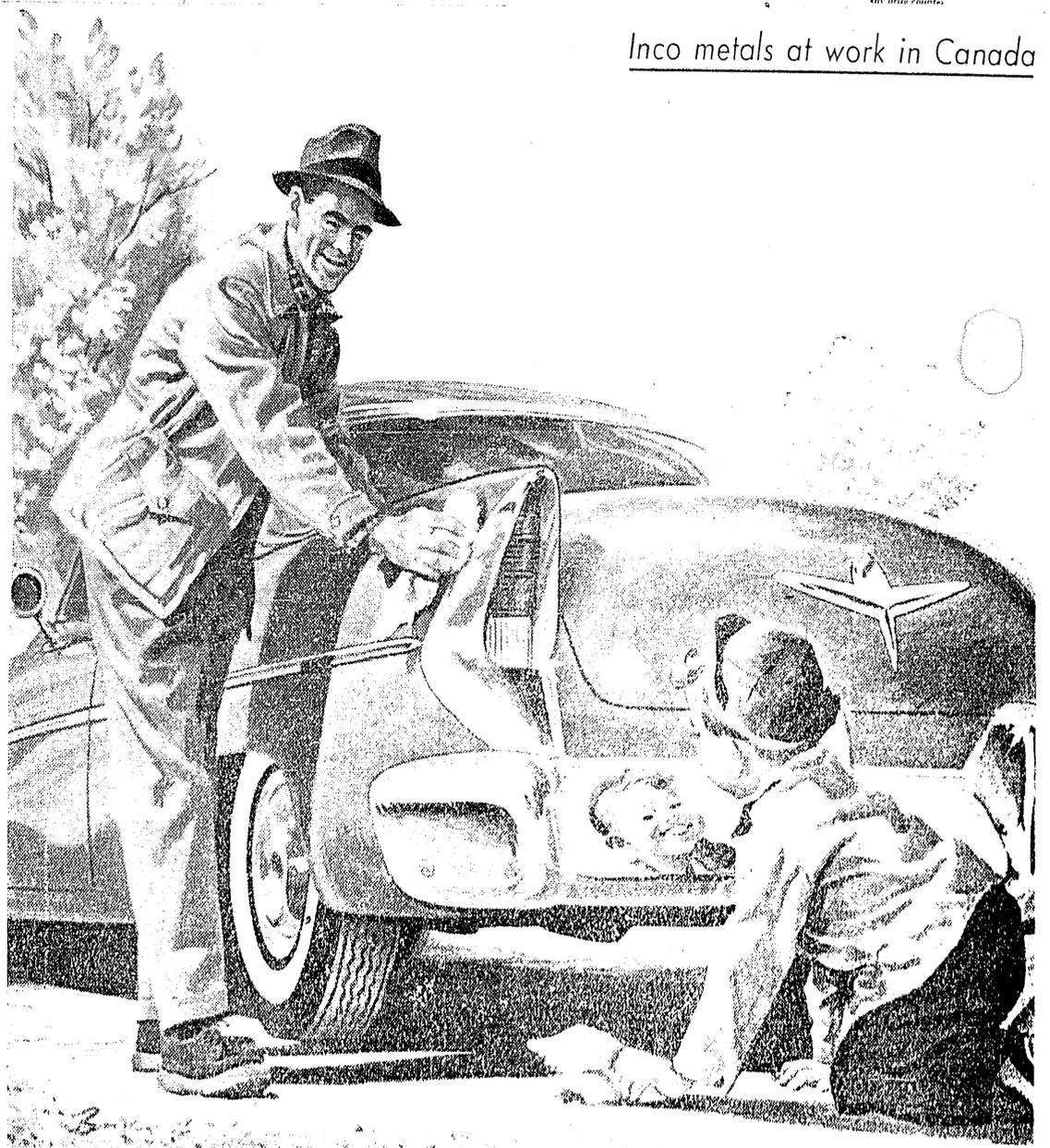
We ordinarily speak of automobile bumpers, grilles, fenders and bright metal trim as being "chrome plated". Actually, these parts are plated with both nickel and chromium. The nickel is the base metal and the chromium is the finish. Inco Nickel is used in the production of these and many other products of Canadian origin for the automobile industry.
